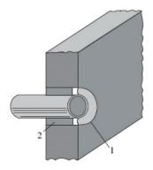
Figure 3: Illustration of centered penetration in a wall.
