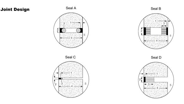
Figure 1: Typical linear joint system design for DOWSIL™ FIRESTOP 700 Sealant.
